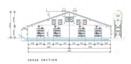
The conveyor belt system is operated every 5 - 7 days with the manure going directly into a parked trailer outside the building. After 14 months the flock is removed and
