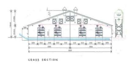
The conveyor belt system is operated every 5 - 7 days and removes approximately 16 tonnes from the internal conveyor belt systems via an external conveyor belt into a
